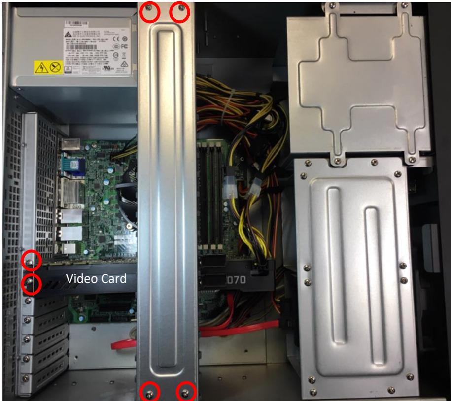
**STEP 3:** Replace cover and reinstall the PC in the cabinet.
